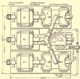
Fig. 274.—Three-cylinder, two-stage turbo-generator unit. Capacity is 60,000 kw.
